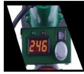
Digital temperature control display
